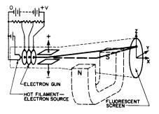
Fig. 12-3. An electron-beam tube.
