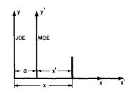
Fig. 11–1. Two parallel coordinate systems.
