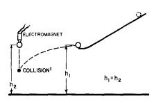
Fig. 7–3. Apparatus for showing the independence of vertical and horizontal motions.
