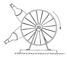
Fig. 44–2. The rubber-band heat engine.
