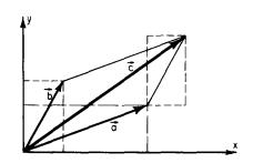
Fig. 11-4. The addition of vectors.
