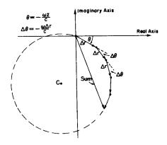
Fig. 30–11. Graphical solution of  $\int_{-\infty}^{\infty} e^{-i\omega r/c} dr$ .
