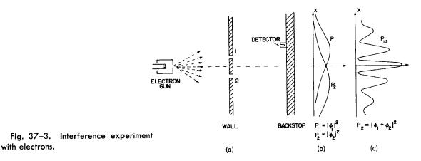
Beyond the wall is another plate which will serve as a "backstop." In front of the backstop we place a movable detector. The detector might be a geiger counter or, perhaps better, an electron multiplier, which is connected to a loudspeaker.
