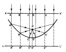
Fig. 26-12. A paraboloidal mirror.
