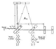
Fig. 15–2. Schematic diagram of the Michelson-Morley experiment.
