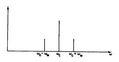
Fig. 48–5. The frequency spectrum of a carrier wave  $\omega_c$  modulated by a single cosine wave  $\omega_m$ .
