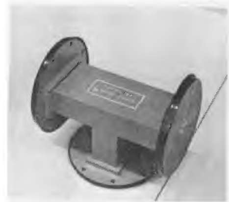
Fig. 24-11. A waveguide "T." (The flanges have plastic end caps to keep the inside clean while the "T" is not being used.)
